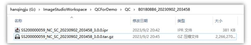
(11) If the auto-uploading function is turned on, the output files (TAR.GZ and IPR) will be automatically uploaded to the selected computer cluster or cloud. Click the "Clear" button to clear the contents, and then drag another image for a new run.
