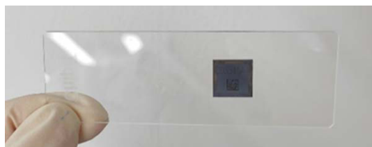
Chip Placement Diagram (backview): Chip number on top, QR code at the bottom.
